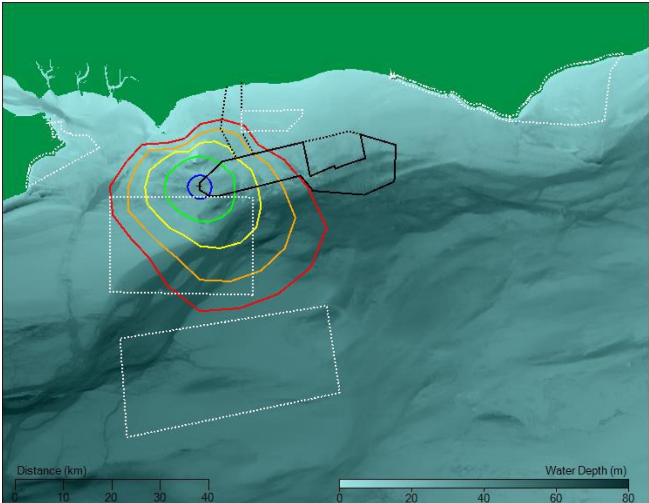
Figure 6 Potential decreases in fish TTS impact ranges using the criteria from Popper et al. (2014) when using various mitigation options, at Western (W) noise modelling location. White dotted lines represent designated MCZs
