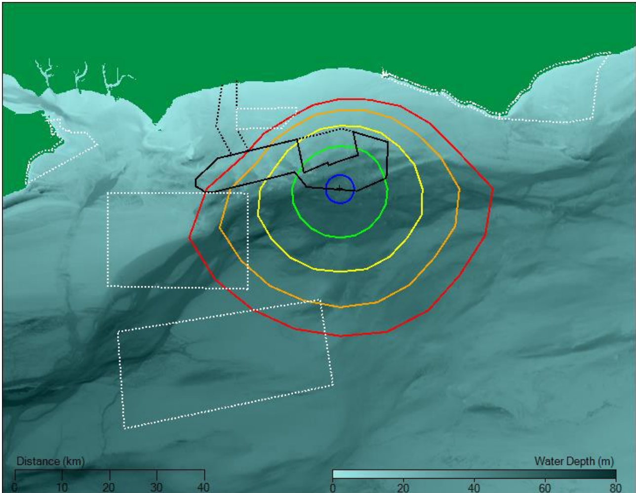
Figure 5 Potential decreases in fish TTS impact ranges using the criteria from Popper et al. (2014) when using various mitigation options, at Southern (S) noise modelling location. White dotted lines represent designated MCZs
